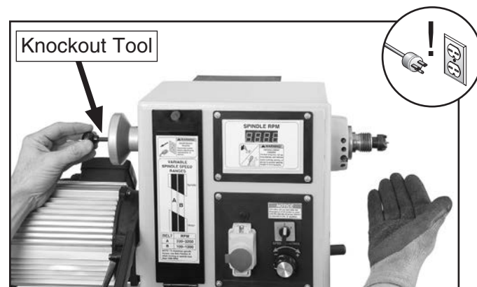
Figure 20. Removing the headstock center.
